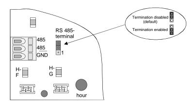
Use a jumper to add a terminal resistor to the RS 485 bus. The jumper must be installed at pins 1 and 2 of the 3-pole plug connector of the RS 485 connector plug (see chapter 1.4).
