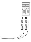
The polarity of the connections is not relevant.
